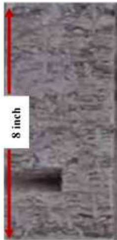
Fig. 3: Close view slabbed core sample, showing burrowed heterolithic sandstone.
