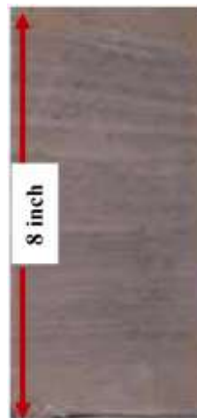
Fig. 7: Close view slabbed core sample at depths of at 4199ft. showing low angle cross-bedded sandstone.
