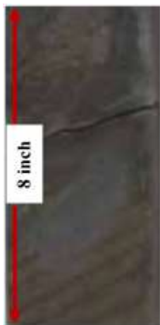
Fig. 10: Close view slabbed core sample, showing cross-laminated siltstone facies.
