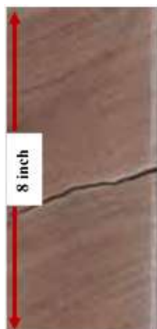
Fig. 6: Close view slabbed core sample, showing cross-bedded sandstone facies.
