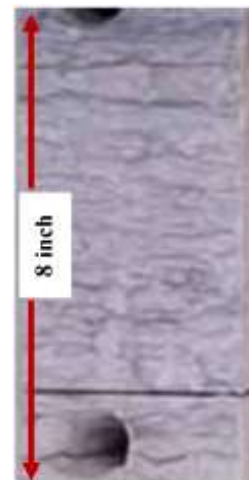
Fig. 5: Close view slabbed core sample, showing burrowed and ripple cross-lamination.
