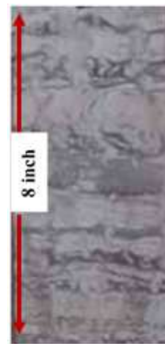
Fig. 2: Close view slabbed core sample, showing parallel to wavy, ripple cross-lamination sandstone and mudstone. This facies comprises very thin to thin bedded sandstone interbedded with thin beds of siltstone or micaceous black mudstone.
